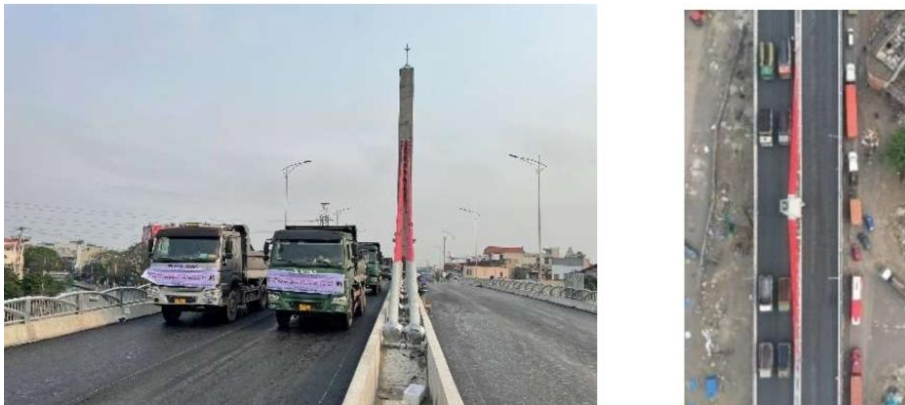
Fig. 9 – Layout diagram of trucks (load on one side of the bridge)
