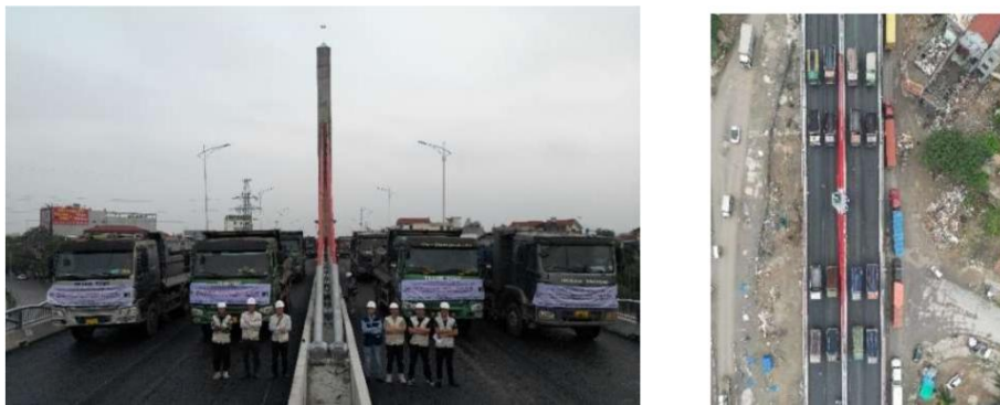
Fig. 8 – Layout diagram of trucks (symmetrical about the bridge's center)
